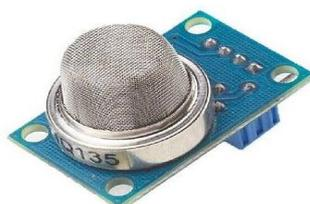
Figure 5. MQ-135 air quality sensor
